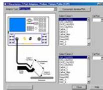
1. One-port cal here using coaxial standards
