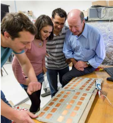
Figure 7: The first tunable metasurface developed at Institut Langevin at 2.45GHz with from right to left Mathias Fink, Matthieu Dupré, Nadège Kaïna and Geoffroy Lerosey (2012).
