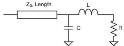
Figure 4 - A graphic representation of the load model
