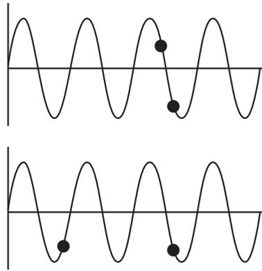
Figure 15: The effect of step size on interpolation is shown here
