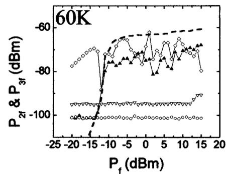
FIG. 3. Power dependence of second- and third-order harmonic generation on both non-GB YBCO surface and GB at 60 K ( $\ll T_c$ ) (filled triangles:  $P_{3f}$  on GB; diamonds:  $P_{2f}$  on GB; circles:  $P_{3f}$  on non-GB; inverted triangles:  $P_{2f}$  on non-GB). The uncoupled ERSJ model calculation for the power dependence of the third-harmonic generation on the grain boundary at 60 K is also plotted as a dashed line for comparison.
