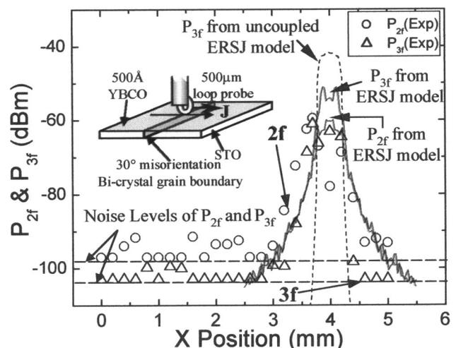
FIG. 4. Second-order ( $P_{2f}$ , circles) and third-order harmonic ( $P_{3f}$ , triangles) power along a line crossing the bicrystal grain boundary, which is located at  $X=4$  mm, with input power  $P_f=+8$  dBm. Calculations of  $P_{2f}$  and  $P_{3f}$  from the coupled ERSJ model are shown in solid lines, and  $P_{3f}$  from the uncoupled ERSJ in a dashed line. Inset is the schematic of the probe-sample arrangement.
