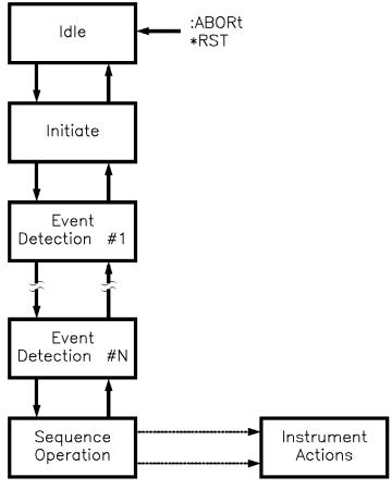
Figure 1-35. Generalized Trigger Model
