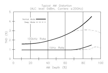
$^{13}$  Deep mode offers reduced distortion for very deep AM. Waveform is DC-coupled and feedback-leveled at ALC levels above -13 dBm. At ALC levels below -13 dBm, output is DC-controllable, but subject to typical sample-and-hold drift of 0.25 dB/second.
