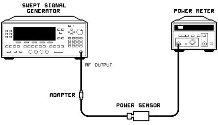
Figure 1-10. Power Sweep and Power Slope Operation
