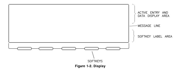
Active Entry and Data Display Area: This area typically displays the frequency and power information of the current instrument state. When data entry is expected, the swept signal generator uses all or part of this area to record the entries. The active entry arrow (-->) indicates the active entry function and its current value.
