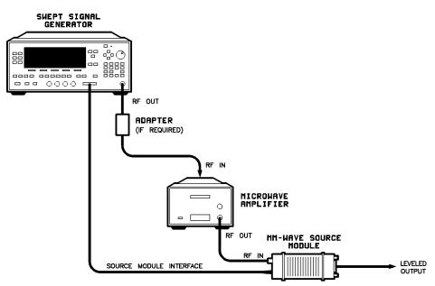
Figure 1-15. MM-wave Source Module Leveling Using a Microwave Amplifier
