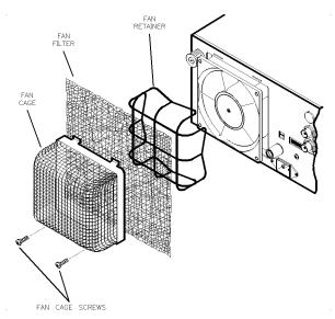
Figure 4-2. Removing the Fan Filter
