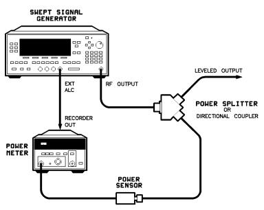
Figure 1-13. Leveling with a Power Meter
