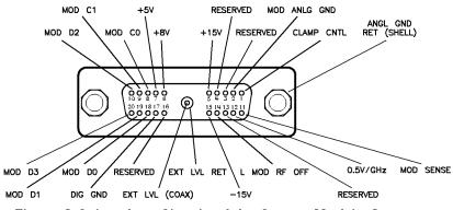
Figure C-3. Interface Signals of the Source Module Connector
