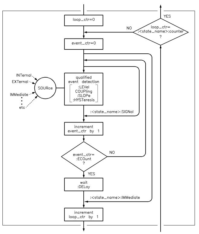
Figure 1-38. Inside an Event Detection State
