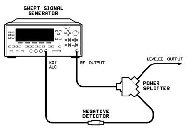
Figure A-2. Typical External Leveling Hookup
