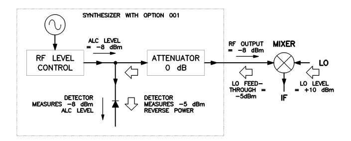
Figure 1-16. Reverse Power Effects, Coupled Operation with -8 dBm Output
