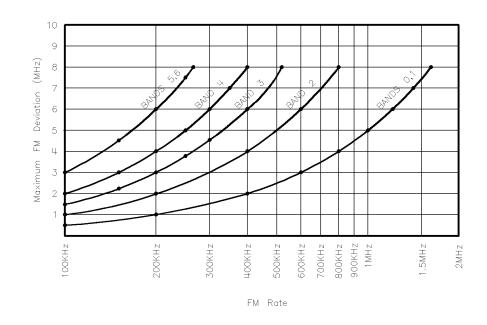
Figure M-3. FM Deviation and Rate Limits
