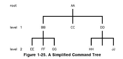
In the command tree shown in Figure 1-25, the command closest to the top is the *root command*, or simply the *root*. Notice that you must follow a particular *path* to reach lower level subcommands. For example, if you wish to access the GG command, you must follow the path AA to BB to GG.
