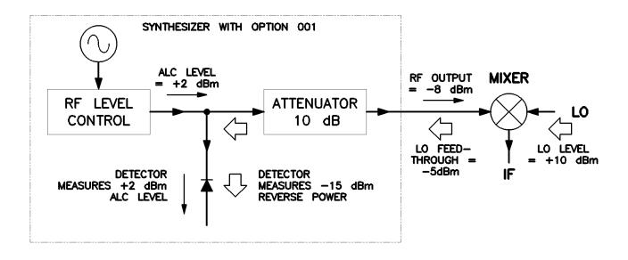
Figure 1-17. Reverse Power Effects, Uncoupled Operation with -8 dBm Output
