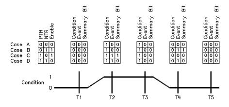
Figure 1-34. Typical Status Register Bit Changes
