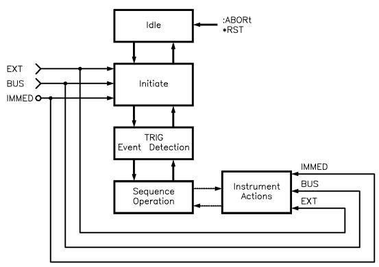
Figure 1-41. The TRIG Trigger Configuration
