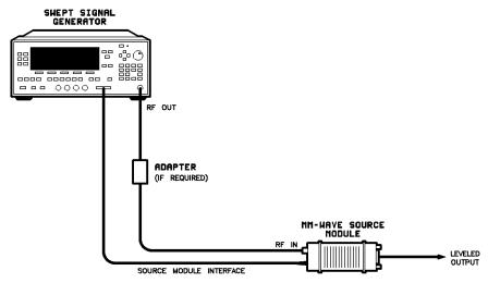
Figure 1-14. MM-wave Source Module Leveling
