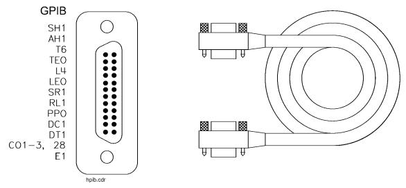
Figure C-2. GPIB Connector and Cable
