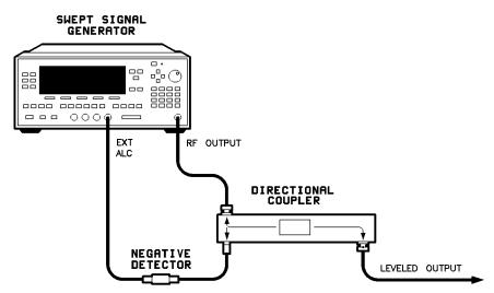
Figure 1-11. ALC Circuit Externally Leveled
