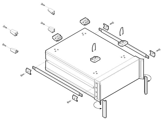
Figure 3-3. Removing the Side Straps and Feet
