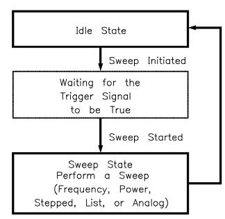
Figure 1-42. 8360 Simplified Trigger Model
