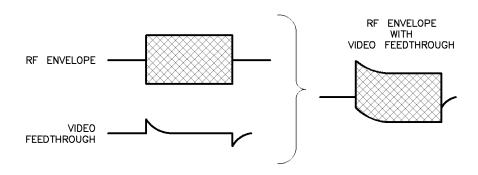
Figure M-6. Video Feedthrough
