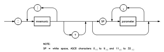
Figure 1-30. Simplified Subsystem Command Syntax
