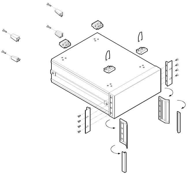
Figure 3-5. Rack Mount Flanges for Swept Signal Generators with Handles Removed
