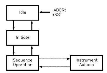
Figure 1-40. The INIT Trigger Configuration
