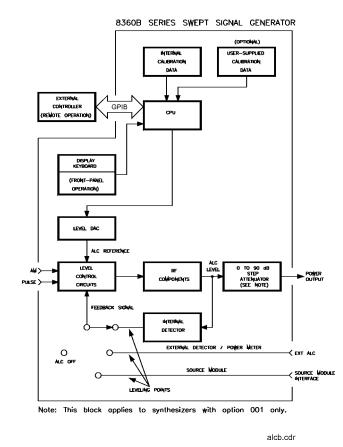
Figure A-1. ALC System Simplified Block Diagram
