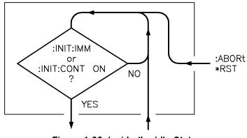
Figure 1-36. Inside the Idle State
