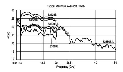
$^3$  Specification applies over the 0 to 35 °C temperature range (0 to 25 °C for output frequencies > 20 GHz). Maximum leveled output power over the 35 to 55 °C temperature range typically degrades by less than 2 dB.
