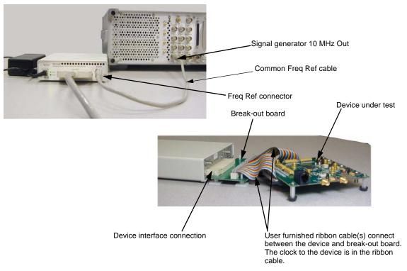
Figure 11-8 Example Setup using the PSG 10 MHz Frequency Reference
