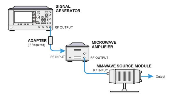
Figure 11-24 Setup for E8267D PSG and E8257D PSG with Option 1EA
