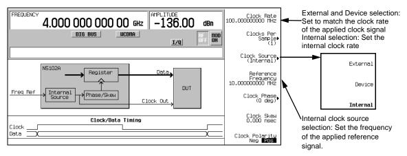
When you select a clock source, you must let the N5102A module know the frequency of the clock signal using the **Clock Rate** softkey. In the internal clock source mode, use this softkey to set the internal clock rate. For device and external clock sources, this softkey must reflect the frequency of the applied clock signal.
