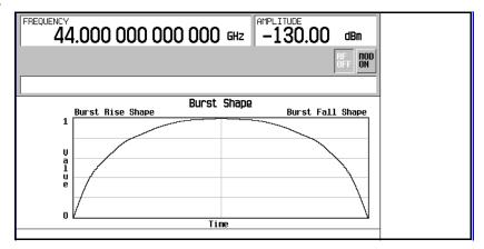
NOTE To return the burst shape to the default conditions, press Return > Return > Confirm Exit From Table Without Saving > Restore Default Burst Shape.
