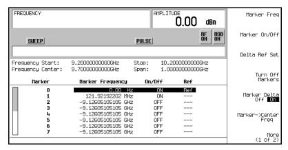
5. Move the cursor back to marker 1 and press Marker Freq. Turn the front panel knob while observing marker 1 on the 8757D.
