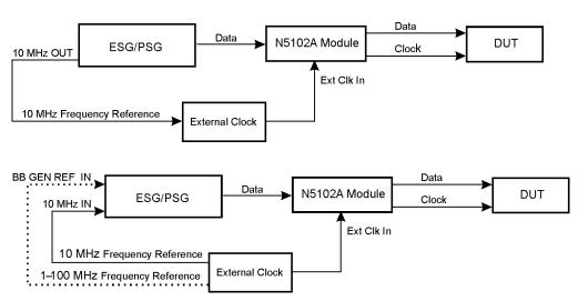
NOTE: Use only one of the two signal generator frequency reference inputs.
