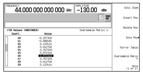
8. For this example, the desired OSR is 4, which is the default, so no action is necessary.
