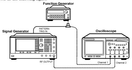
This connection is applicable to all external triggering methods. The optional oscilloscope connection enables you to see the effect that the trigger signal has on the RF output.
