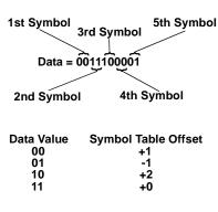
When applied to the user-defined default 4QAM I/Q map, starting from the 1st symbol (data 00), the differential encoding transitions for the data stream (in 2-bit symbols) 0011100001 appear in the previous illustration.
