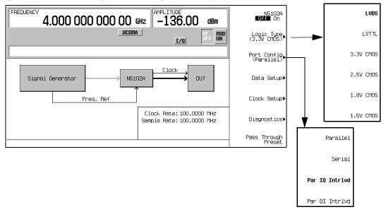
Refer to Figure 11-10. Press the Logic Type softkey.
