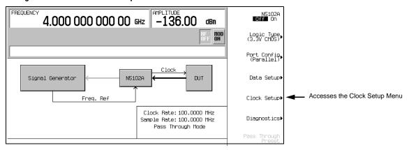
From this softkey menu, set all of the clock parameters that synchronize the data between the N5102A module and the device. From this menu, the clock signal phase can be changed so the clock occurs during the valid portion of the data. Figure 11-18 shows the clock setup menu.
