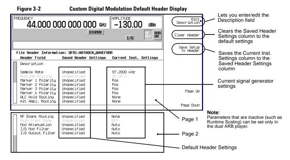
2. Save the information in the Current Inst. Settings column to the file header: Press Save Setup To Header.
