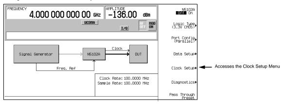
From this softkey menu, set all of the clock parameters that synchronize the clocks between the N5102A module and the PSG. You can also change the clock signal phase so the clock occurs during the valid portion of the data. Figure 11-14 shows the clock setup menu.
