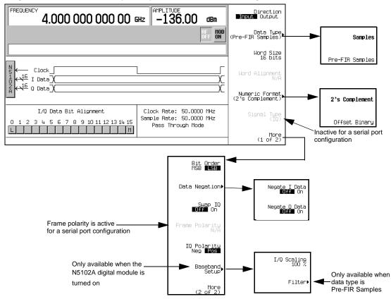
Figure 11-20 Data Setup Softkey Menu with Parallel Port Configuration
