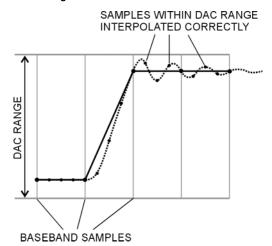
Although scaling maintains the basic shape of the waveform, too much scaling can compromise its integrity because the bit resolution can be so low that the waveform becomes corrupted with quantization noise. Maximum accuracy and optimum dynamic range are achieved by scaling the waveform just enough to remove the DAC over-range error. Optimum scaling varies with waveform content.
