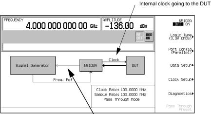
Line is grayed out until the N5102A module interface is turned on
