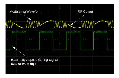
**NOTE** In the real-time Custom mode, the behavior is reversed: when the gating signal is *high*, you see the modulated waveform.
