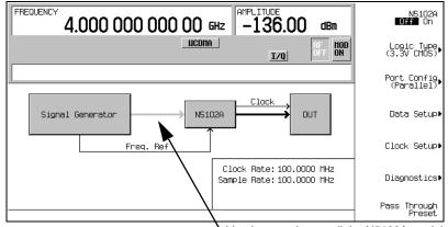
Line is grayed out until the N5102A module interface is turned on
