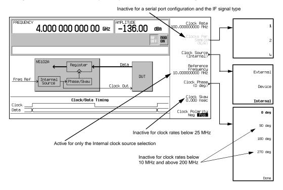
The top graphic on the display shows the current clock source that provides the output clock signal at the Clock Out and Device Interface connectors. The graphic changes to reflect the clock source selection discussed later in this procedure. The bottom graphic shows the clock position relative to the data. The displayed clock signal will change to reflect the following:
