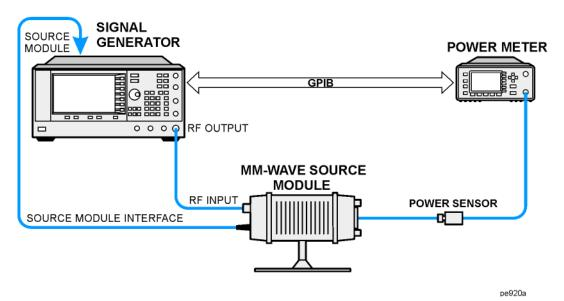
NOTE To ensure adequate RF amplitude at the mm-wave source module RF input when using Option 1EA signal generators, maximum amplitude loss through the adapters and cables connected between the signal generator's RF output and the mm-wave source module's RF input should be less than 1.5 dB.
