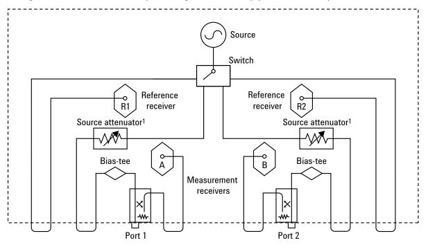
1. Source attenuator for E8362/3/4B is 60 dB in 10 dB steps. Source attenuator for E8361A is 50 dB in 10 dB steps.
