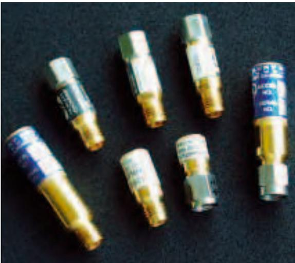
1: Travelling standards: Three attenuators (top) and four terminations (below) with coaxial 2.4 mm connectors.
