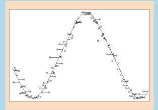
**Figure 6.** The circles show the sampled signal and the solid curve shows the estimated signal. The horizontal bars show the differences between the times estimated from the curve and the nominal oscilloscope timebase. (From [4].)
