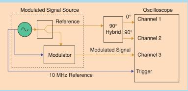
**Figure 5.** A typical measurement configuration used for characterizing a modulated signal with the NIST's Timebase Correction Software [31].
