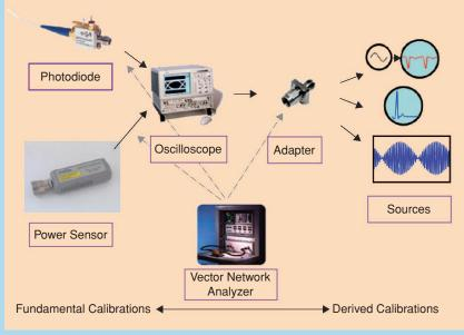
**Figure 2.** The NIST waveform traceability chain.
