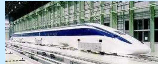
The Yamanashi MLX01 MagLev test vehicle achieved a speed of 343 mph (552 kph) on April 14, 1999
