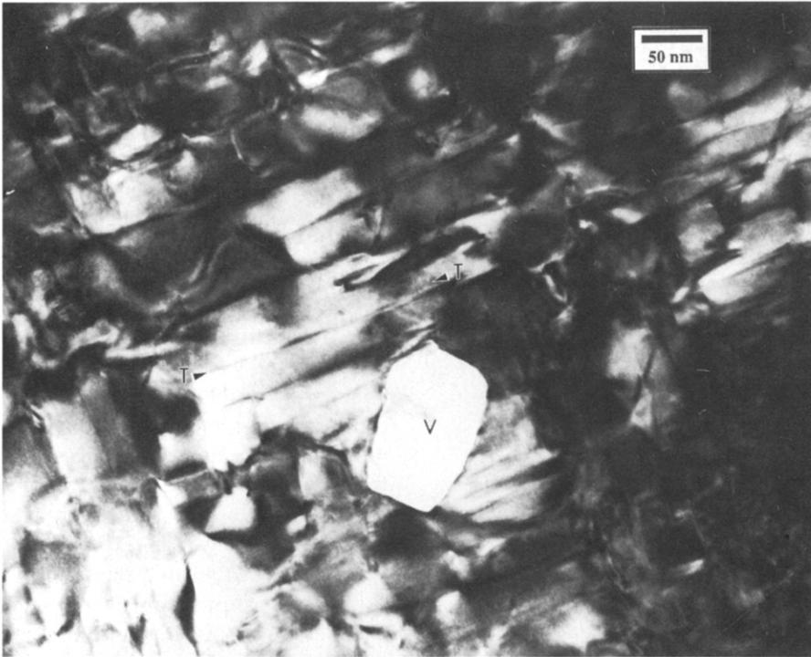
Fig. 9. Microstructure of a *c*-axis YBCO film on MgO (film #123A5). A void, marked "V", near the center of the micrograph is an uncommon feature. Twin boundaries are visible as dark lines, with an example marked with "T"s.
