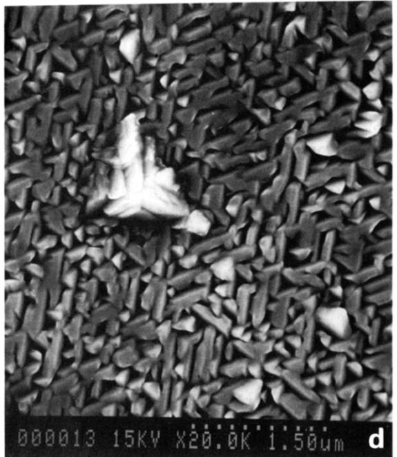
Fig. 4. SEM micrographs of differently textured YBCO thin films on different substrates. (a) *c*-axis oriented film on MgO, (b) *a*-axis oriented films on SrTiO<sub>3</sub> (100), (c) (103) oriented films on SrTiO<sub>3</sub> (100) and (d) (113) oriented films on SrTiO<sub>3</sub> (111).
