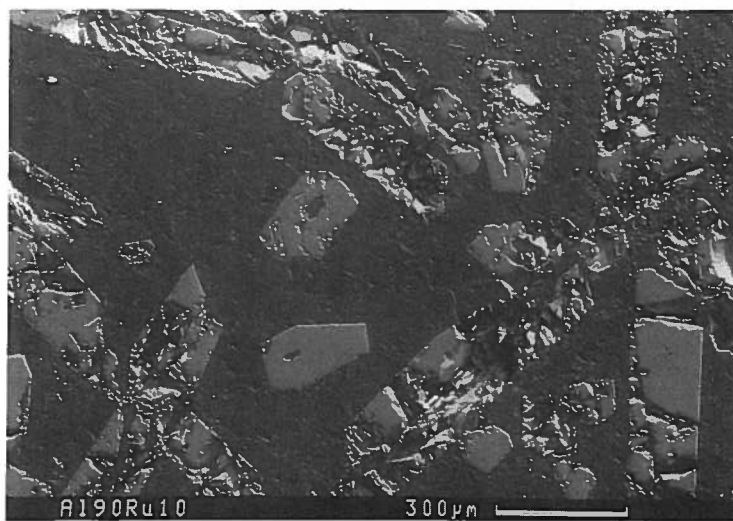
Fig. 4. SEM micrograph showing the structure of \text{Al}_{90}\text{Ru}_{10} after cooling in the calorimeter at the rate of 20 \text{ K min}^{-1} ; the angular crystals are \text{Al}_{13}\text{Ru}_4 and the matrix is eutectic \text{Al} + \text{Al}_6\text{Ru} .
