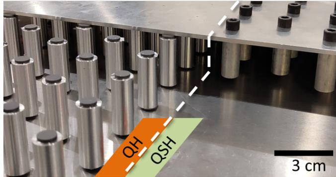
Figure G.3: An open-plate view of the QH-QSH interface 2-port isolator experimental set-up. Note that the biasing magnets on the QH region are not shown.
