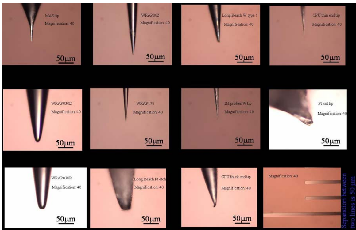
Fig. 2.23: All of the tips investigated for use in the combined NSMM/STM microscope, imaged in an optical microscope with magnification 40 for the objective lens.
