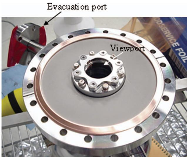
FIG. 7. Picture of the interface flange with viewport at the center.
