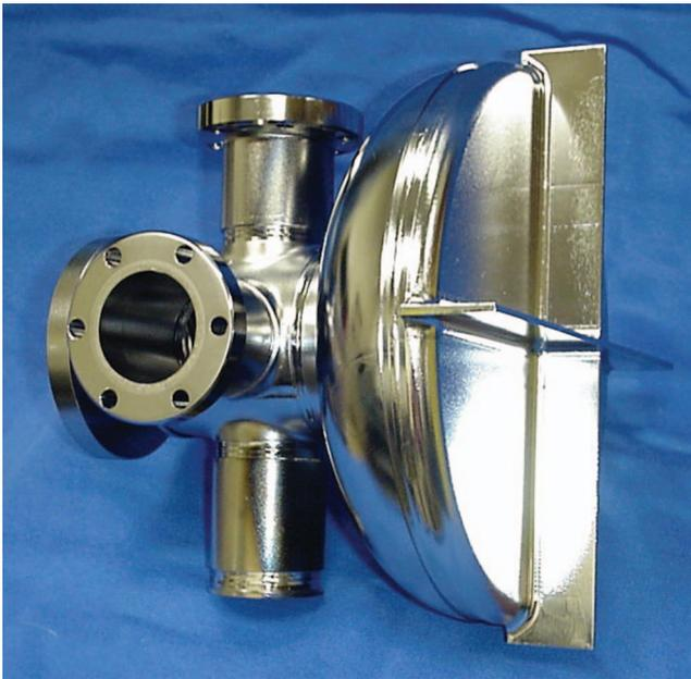
FIG. 2. Picture of the SRF niobium cavity.
