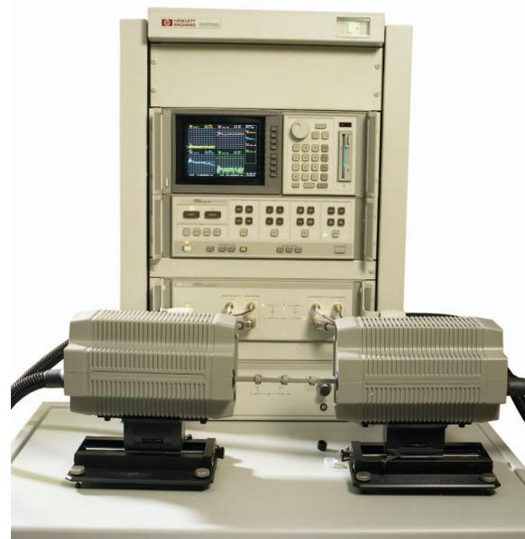
**Figure 2.** A coaxial mm-wave measurement bench based on the Agilent 8510 VNA. This analyzer was the industry reference for microwave measurements for many years.
