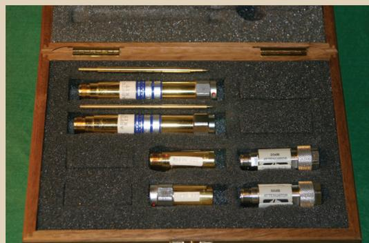
**Figure A.** Type-N travelling standards used for the ARFTG MCP.
