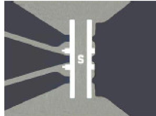
Figure 2: Images showing correct alignment and placement of probe tips of both ACP and Infinity style probes.
