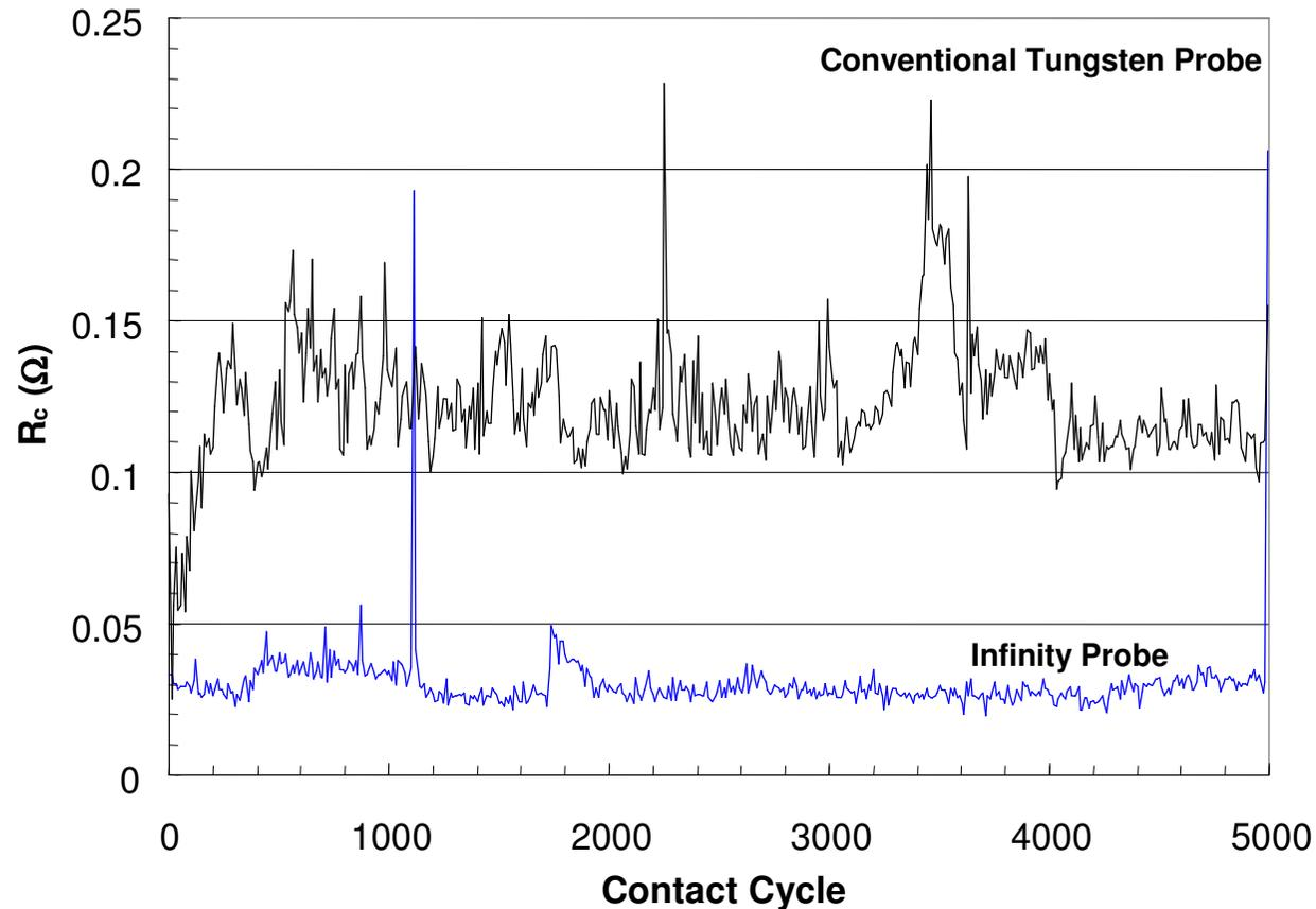
Contact resistance on un-patterned aluminum averages about 30 m $\Omega$  over 5000 contact cycles at ambient
