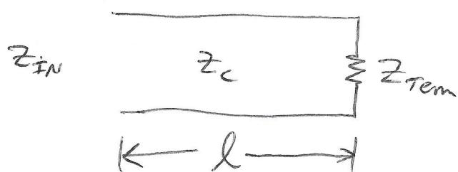
$$\bar{z}_{in} = \frac{\bar{z}_{Term} + i \tan \beta l}{1 + i \bar{z}_{Term} \tan \beta l} \quad \bar{z} = z/z_c$$
