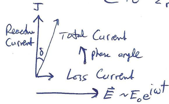
$$\begin{aligned} \tan \delta &= \frac{\text{Loss Current}}{\text{Reactance Current}} \\ &= \epsilon_r'' / \epsilon_r' \end{aligned}$$
