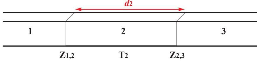
Figure 2.7: Setup of the three-layer transfer matrix model inside a waveguide. The layers are labeled 1, 2, 3, with the associated impedance matrix,  $Z_{ij}$ , and transmission matrix,  $T_k$ , where  $i, j, k$  refer to a specific layer. Layers 1 and 3 extend to infinity, while layer 2 has thickness  $d_2$ .
