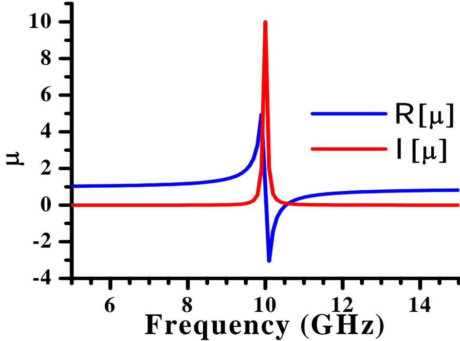
Figure 2.6: A plot of the real part of the permeability,  $\Re[\mu]$ , shown in blue, and the imaginary part of the permeability,  $\Im[\mu]$ , shown in red, versus frequency. The values used to generate this plot were  $f = 0.1$ ,  $\omega_0 = 2\pi \times 10$  GHz, and  $\Gamma = 2\pi \times 0.1$  GHz, in Equation (2.97).
