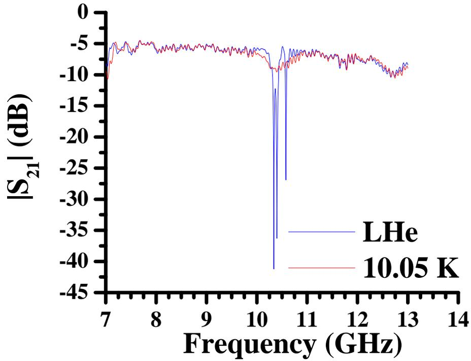
Figure 5.6: A plot of the electromagnetic transmission,  $|S_{21}|$ , versus frequency for an array of 3 Nb split-ring resonators, inside the Ag-plated brass X-band waveguide. The blue curve is data taken while the Ag-plated brass X-band waveguide and Nb split-ring resonators were immersed in liquid Helium, denoted LHe, while the red curve is data that was taken at 10.05 K.
