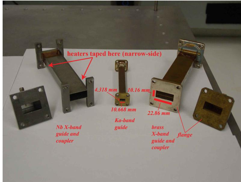
Figure 3.5: Waveguides used in the experiments, with inner dimensions specified. From left to right: *X*-band Nb waveguide-to-coaxial cable coupler; *X*-band Nb waveguide; *Ka*-band waveguide; Ag-plated brass *X*-band waveguide; *X*-band brass waveguide-to-coaxial cable coupler.
