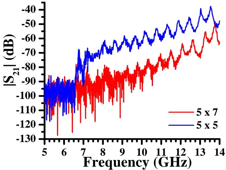
Figure 4.10: A plot of the electromagnetic transmission,  $|S_{21}|$ , versus frequency for a Nb wire array in the Ag-plated brass X-band waveguide. The red curve corresponds to an array of five wires transverse and seven wires deep, while the blue curve is data taken for a Nb wire array with five wires transverse and five wires deep. In both cases, the wires were symmetric with respect to the center of the Ag-plated brass X-band waveguide, and the waveguide was immersed in liquid Helium.
