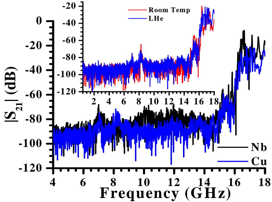
Figure 4.9: A plot of the electromagnetic transmission,  $|S_{21}|$ , versus frequency for the Ag-plated brass X-band waveguide immersed in liquid Helium, with a Nb wire array (black curve) and a Cu wire array (blue curve). In all cases, the lattice parameter was  $a = 5.08$  mm. *Inset:* The Cu wire array data at room temperature (red curve) and immersed in liquid Helium (blue curve), abbreviated as LHe.
