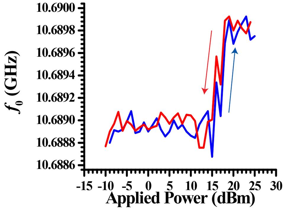
Figure 5.16: A plot of the resonant frequency,  $f_0$ , versus applied power for the single Nb split-ring resonator- $\beta$ , inside the Ag-plated brass X-band waveguide, immersed in liquid Helium. The power is measured after the amplifier, but before entering the waveguide, as shown in Figure (3.14). The blue curve is increasing power, and the red curve is decreasing power.
