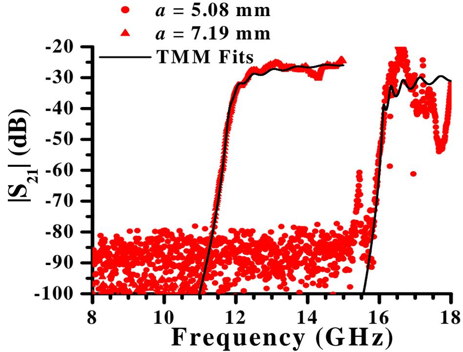
Figure 4.7: A plot of the electromagnetic transmission,  $|S_{21}|$ , versus frequency for a Nb wire array in the Ag-plated brass X-band waveguide at room temperature. The red circles are the data for the lattice parameter of  $a = 5.08$  mm, while the red triangles are the data for the lattice parameter of  $a = 7.19$  mm. The black curves are the fits from the three-layer transfer matrix model.
