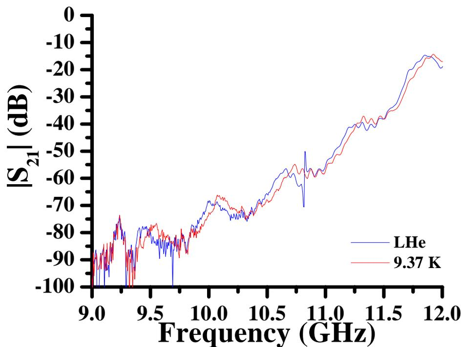
Figure 6.6: A plot of the electromagnetic transmission,  $|S_{21}|$ , versus frequency for the single Nb split-ring resonator- $\gamma$  in a Nb wire array measuring five wires transversely, and thirteen wires longitudinally, with a lattice parameter of  $a = 7.19$  mm, in the Ag-plated brass X-band waveguide. The blue curve was measured in liquid Helium, denoted as LHe, and the red curve was measured at 9.37 K.
