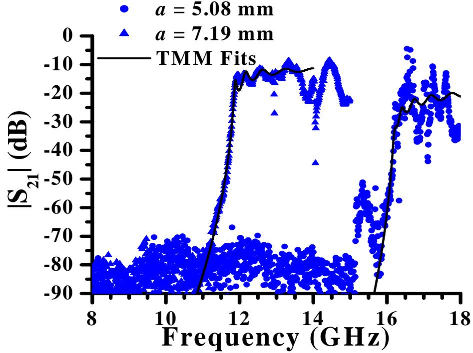
Figure 4.6: A plot of the electromagnetic transmission,  $|S_{21}|$ , versus frequency for a Nb wire array in the Ag-plated brass X-band waveguide at a temperature of 7 K. The blue circles are the data for the lattice parameter of  $a = 5.08$  mm, while the blue triangles are the data for the lattice parameter of  $a = 7.19$  mm. The black curves are the fits from the three-layer transfer matrix model.
