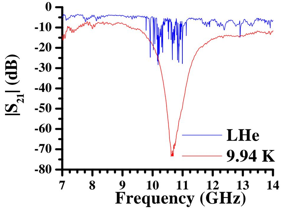
Figure 5.3: A plot of the electromagnetic transmission,  $|S_{21}|$ , versus frequency for an array of 108 Nb split-ring resonators, measured in liquid Helium, denoted by the blue curve and labeled LHe, and at 9.94 K, denoted by the red curve, in the Ag-plated brass X-band waveguide. Rohacell® HF was used to orient the Cu-Ni-Au split-ring resonators.
