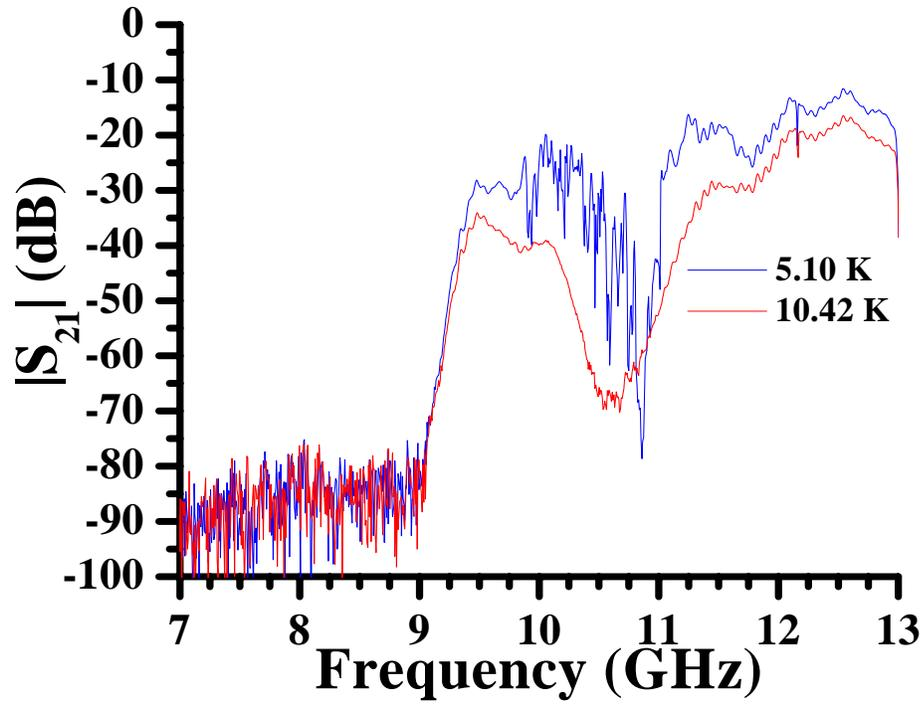
Figure 6.4: A plot of the electromagnetic transmission,  $|S_{21}|$ , versus frequency for an array of 216 Nb split-ring resonators in a Nb wire array measuring five wires transversely and eighteen wires longitudinally, with a lattice parameter of  $a = 7.19$  mm. The blue curve was measured at 5.10 K and the green curve was measured at 10.42 K. The distance separating the wires and Nb split-ring resonator was approximately  $d = 2.54$  mm.
