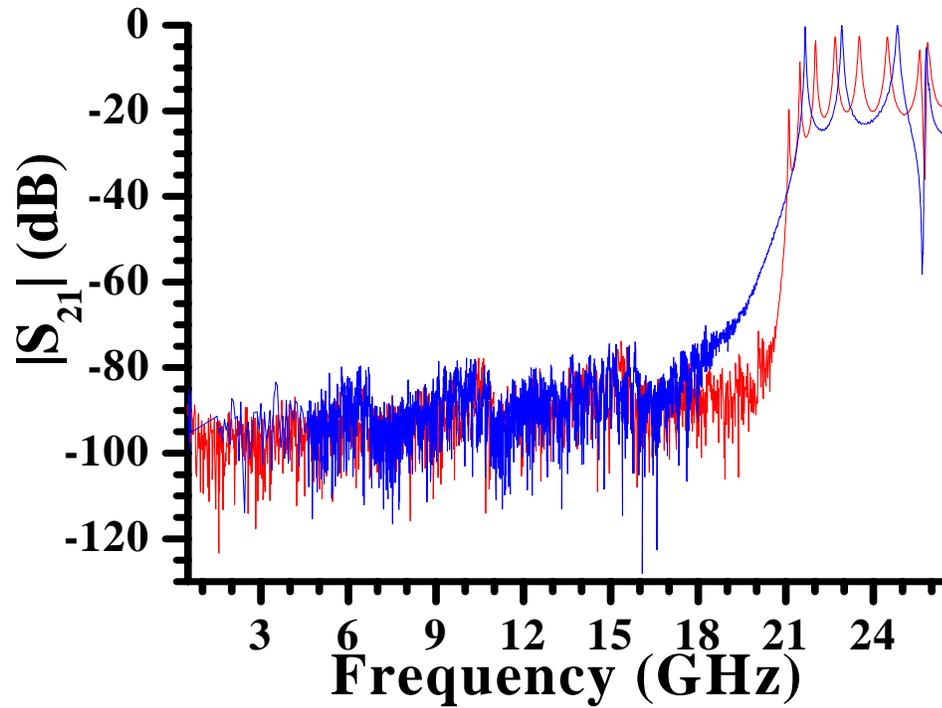
Figure 4.4: A plot of the electromagnetic transmission,  $|S_{21}|$ , versus frequency for an empty *Ka*-band waveguide. The red curve is data taken from the waveguide-to-coaxial cable couplers plus a waveguide that was at least 25 mm in length and at most 100 mm in length, while the blue curve is data taken for the case where the waveguide-to-coaxial cable couplers are directly coupled. The data for both curves were taken at room temperature.
