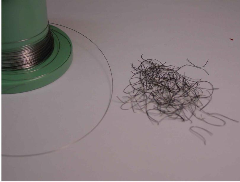
Figure 3.1: *Left:* A spool of the Nb wire. *Right:* Spent Nb wire after removal from a waveguide.
