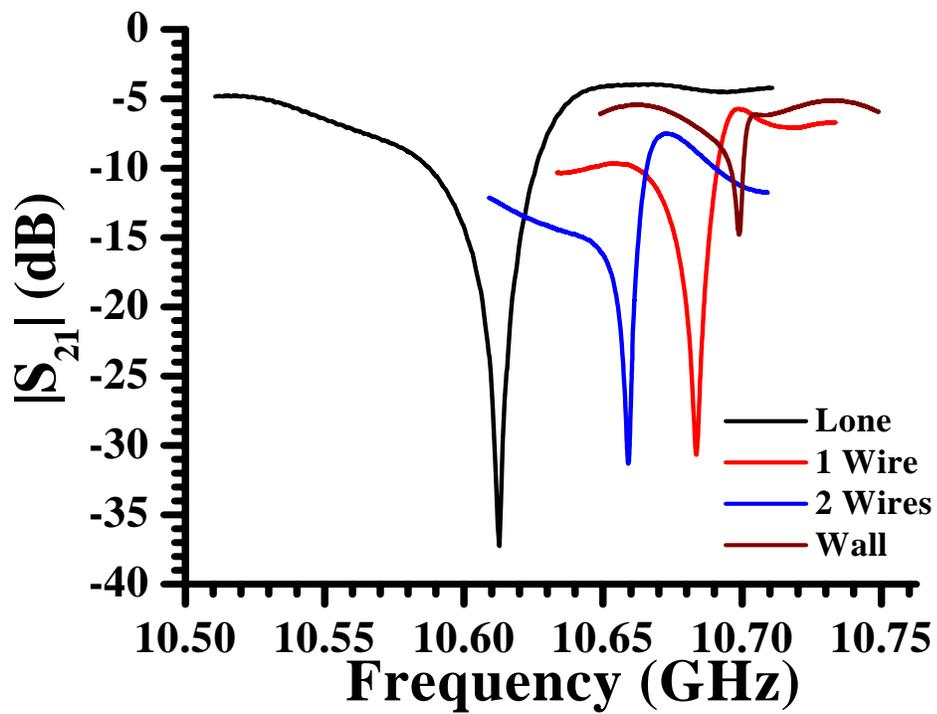
Figure 5.24: A plot of the electromagnetic transmission,  $|S_{21}|$ , versus frequency for the single Nb split-ring resonator  $-\beta$  in an otherwise empty Nb X-band waveguide, with various perturbations. All Nb split-ring resonator orientations were plane-parallel gap-orthogonal.
