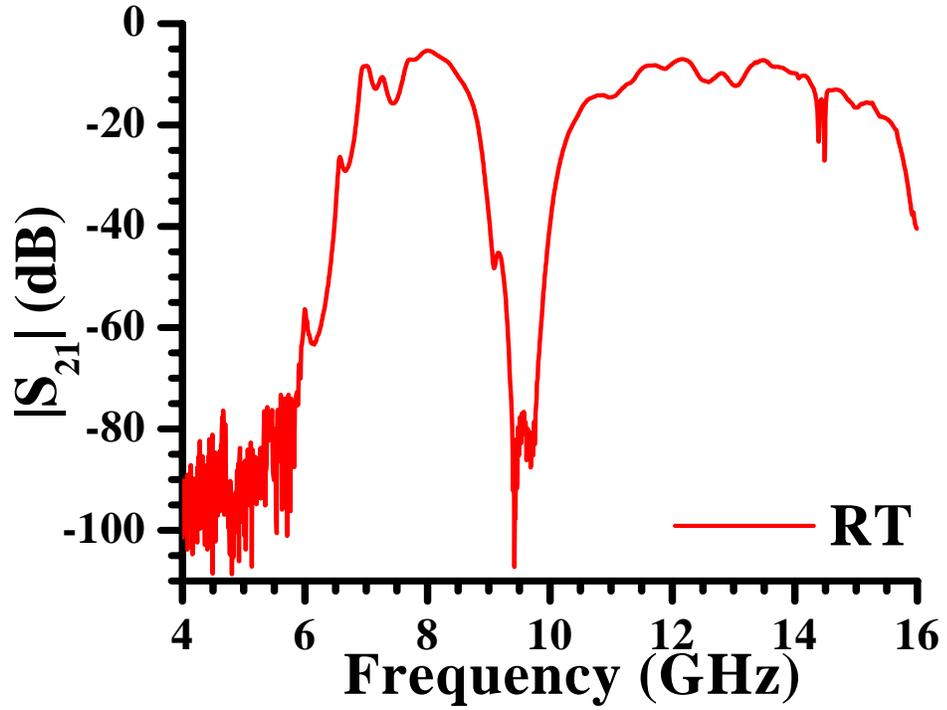
Figure 5.1: A plot of the electromagnetic transmission,  $|S_{21}|$ , versus frequency for an array of 216 Cu-Ni-Au split-ring resonators, measured at room temperature, abbreviated as RT in the figure, in the Ag-plated brass X-band waveguide. Rohacell® HF was used to orient the Cu-Ni-Au split-ring resonators.
