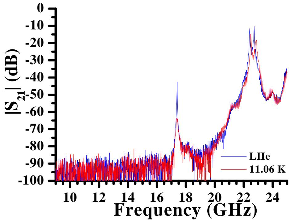
Figure 6.13: A plot of the electromagnetic transmission,  $|S_{21}|$ , versus frequency for a single Nb split-ring resonator in the  $Ka$ -band waveguide, measured in liquid Helium, shown as the blue curve, and 11.06 K, shown as the red curve.
