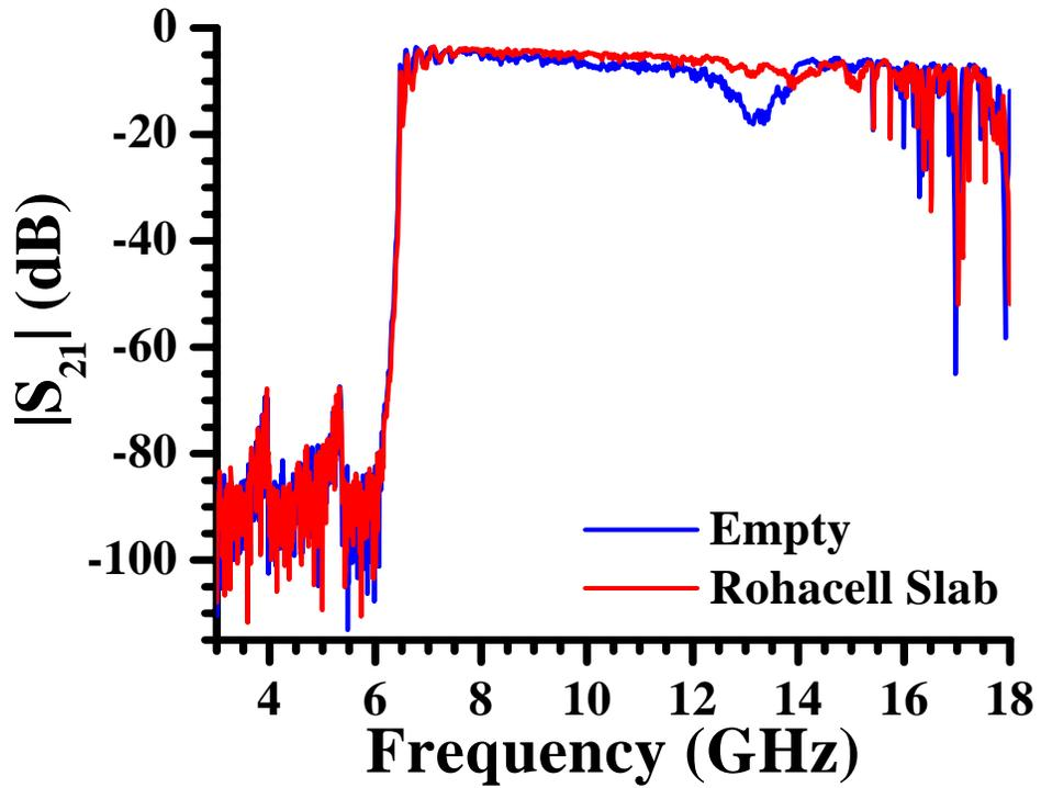
Figure 4.1: A plot of the electromagnetic transmission,  $|S_{21}|$ , versus frequency for an empty Ag-plated brass  $X$ -band waveguide (blue curve), and a Ag-plated brass  $X$ -band waveguide with a  $22.86 \times 10.16 \times 69 \text{ mm}^3$  slab of Rohacell® HF inside (red curve). Both sets of data were taken while the Ag-plated brass  $X$ -band waveguide was immersed in liquid Helium.
