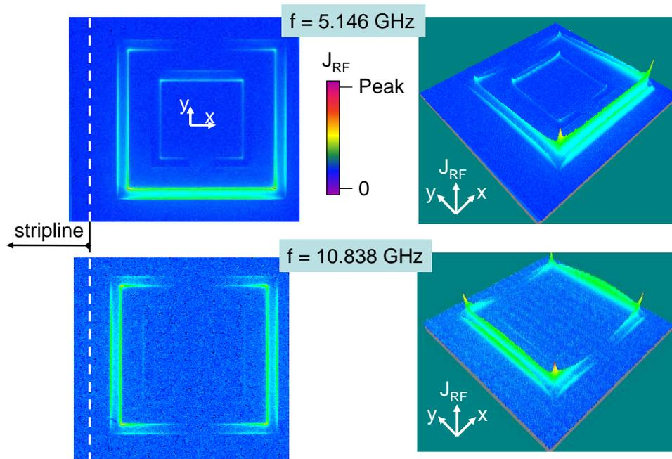
Figure 5.18: A plot of the photoresponse of a  $\text{YBa}_2\text{Cu}_3\text{O}_{7-\delta}$  split-ring resonator. (a): Outer ring resonance at 5.146 GHz; (b): Outer ring resonance at 10.838 GHz. (c) and (d): Three dimensional plots of (a) and (b), respectively.
