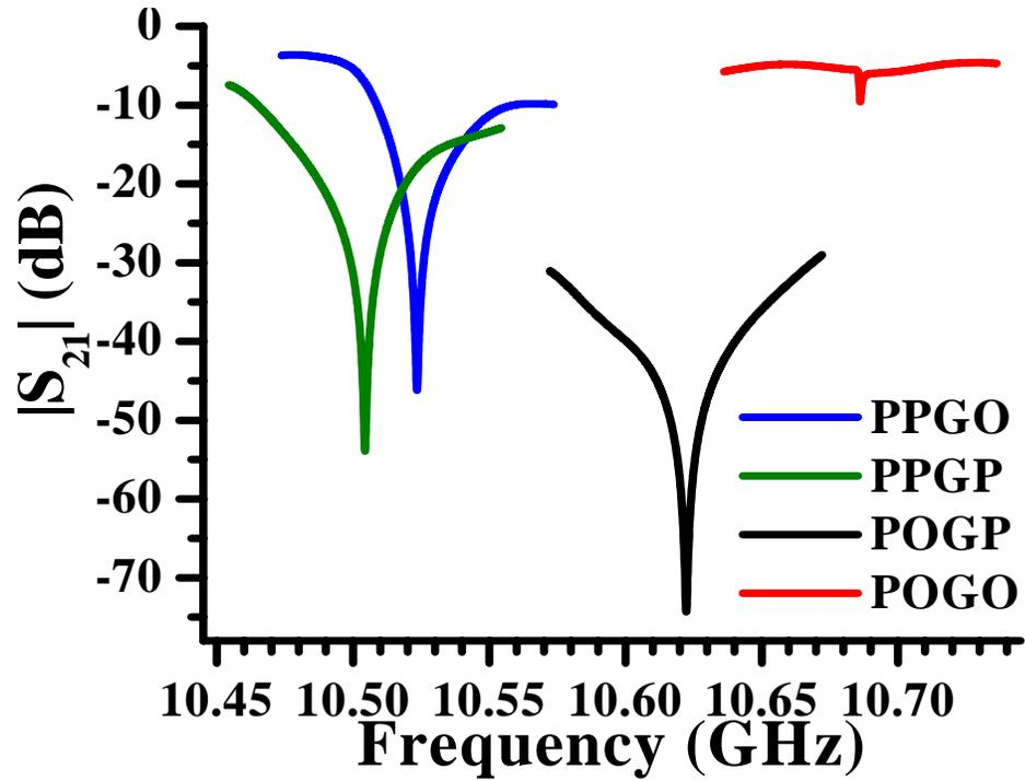
Figure 5.21: A plot of the electromagnetic transmission,  $|S_{21}|$ , versus frequency for the single Nb split-ring resonator- $\pi$ , inside the Nb  $X$ -band waveguide immersed in liquid Helium. The curves are labeled as follows: PPGO (blue): plane-parallel gap-orthogonal; PPGP (green): plane-parallel gap-parallel; POGP (black): plane-orthogonal gap-parallel; POGO (red): plane-orthogonal gap-orthogonal. The orientations were described in Figure (2.10).
