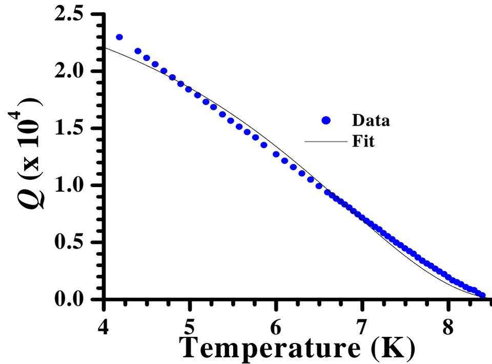
Figure 6.10: A plot of the quality factor,  $Q$ , versus temperature for the single Nb split-ring resonator- $\alpha$  in a Nb wire array measuring five rows transversely and seven rows longitudinally, as in Figure (6.8), inside the Nb X-band waveguide. The blue dots are the data, while the black curve is a fit using Equation (2.161).
