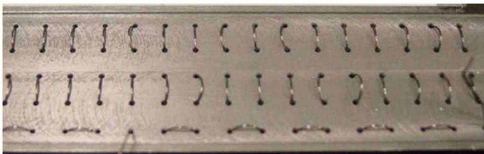
Figure 3.9: A Nb wire array in the Nb  $X$ -band waveguide, with a lattice parameter of  $a = 4.57$  mm. The short lattice parameter prevented the wires from being pulled straight, and forced the wires inside the Nb  $X$ -band waveguide to be curved, as shown in the top of the figure. The bottom of the figure shows a view of the broadside of the Nb  $X$ -band waveguide from the outside.
