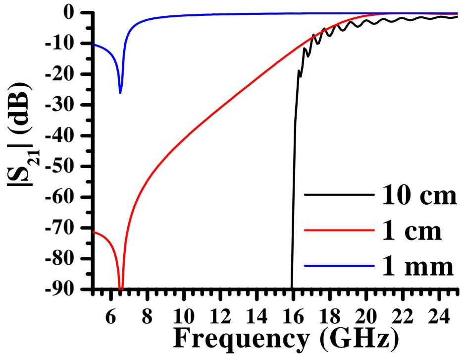
Figure 4.11: A plot of the electromagnetic transmission,  $|S_{21}|$ , calculated from the three-layer transfer matrix model with a plasmalike permittivity, versus frequency for various medium lengths. The black curve is a medium 10 cm in length, the red line a medium 1 cm in length, and the blue curve a medium 10 mm in length. The parameters used to calculate these curves were  $\omega_p = 2\pi \times 16$  GHz, and  $\gamma = 2\pi \times 100$  MHz.
