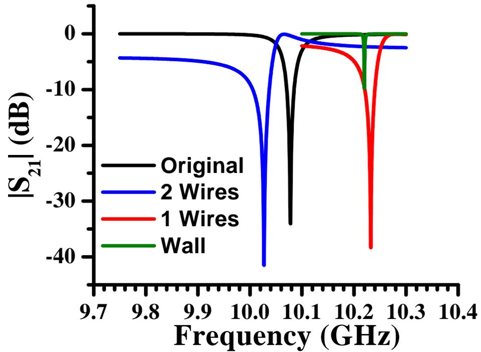
Figure 5.25: A plot of the electromagnetic transmission,  $|S_{21}|$ , versus frequency for a simulation of a single perfect electric conductor splitting resonator in an otherwise empty  $X$ -band waveguide, with various perturbations.
