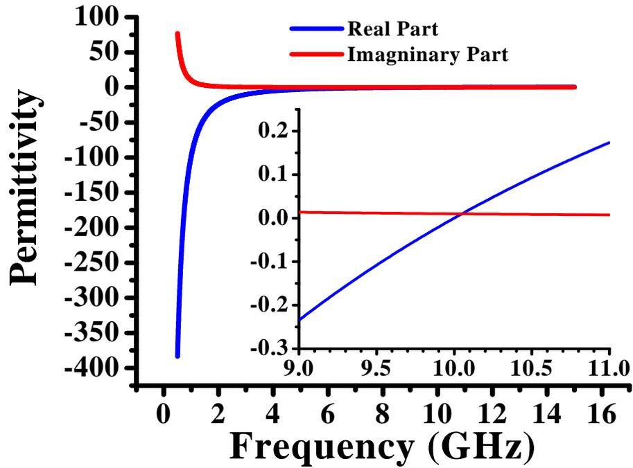
Figure 2.1: A plot of the permittivity of a plasma with a plasma frequency of  $\omega_p = 2\pi \times 10$  GHz and loss parameter of  $\gamma = 2\pi \times 0.1$  GHz. The blue curve is the real part of the permittivity, and the red curve is the imaginary part of the permittivity. The inset shows a close-up of the larger plot in the vicinity of the plasma frequency,  $\omega_p$ .
