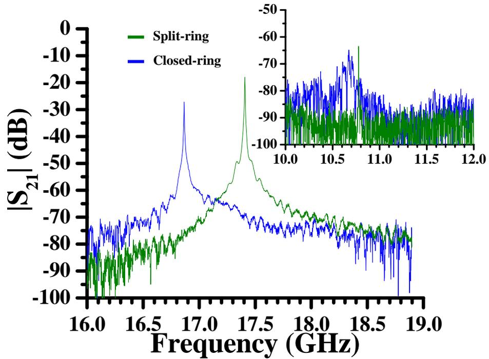
Figure 6.15: A plot of the electromagnetic transmission,  $|S_{21}|$ , versus frequency for the single Nb split-ring resonator- $\pi$ , shown as the green curve, and a single Nb closed-ring resonator, shown as blue curve, in the  $Ka$ -band waveguide-to-coaxial cable couplers, measured in liquid Helium. The main figure is the second harmonic of the current density, and the inset is the fundamental mode of the current density.
