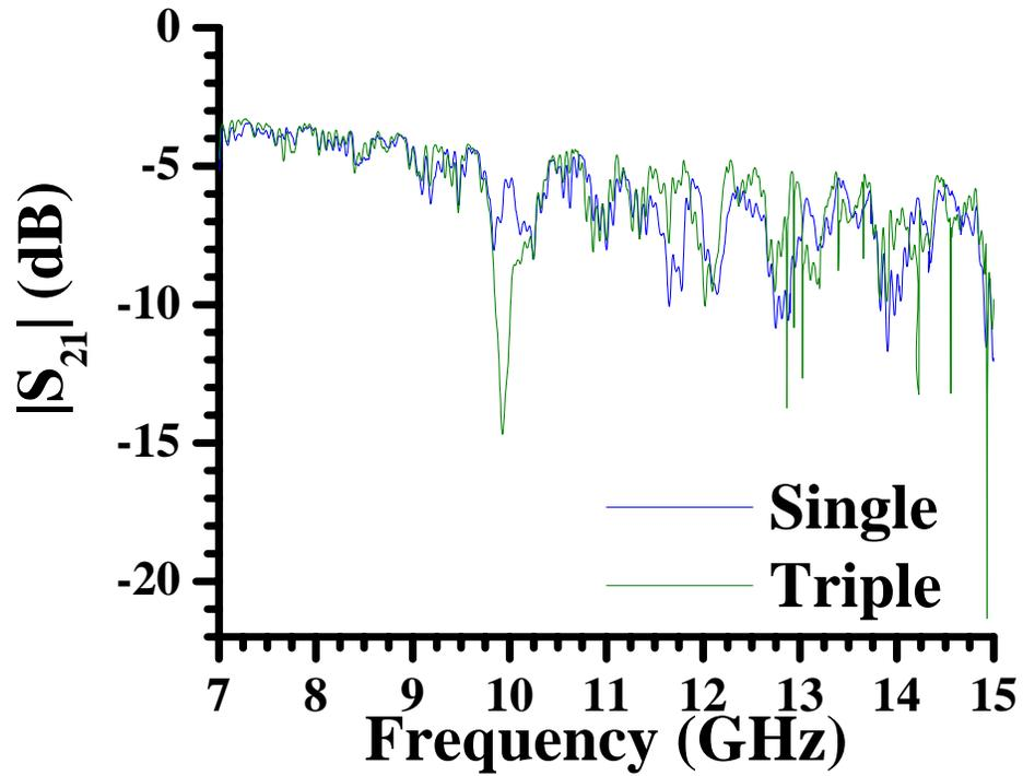
Figure 5.20: A plot of the electromagnetic transmission,  $|S_{21}|$ , versus frequency for an array of a single Cu-Ni-Au split-ring resonator, shown in blue, and three Cu-Ni-Au split-ring resonators, shown in green. The data were measured in the Ag-plated brass X-band waveguide with the Nb waveguide-to-coaxial cable couplers. The ringing in the data were due to standing waves in the coaxial cables, due to impedance mismatches in the entire circuit.
