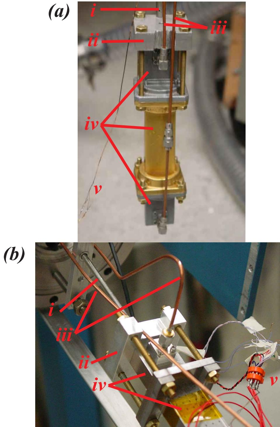
Figure 3.11: The experimental probes. (a) Small Dewar probe. (b) Large Dewar probe. Both figures contain numbers that refer to the same features: (i) support rod; (ii) Al block; (iii) coaxial cables; (iv) waveguide and couplers; (v) thermometer (and heater for (b)).
