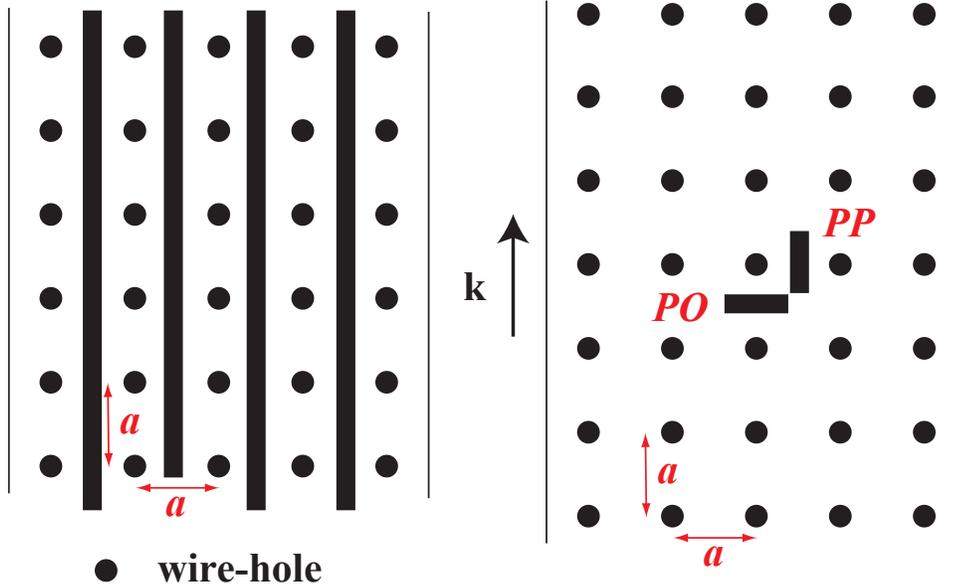
Figure 3.10: A metallic wire array, shown as black circles with lattice parameter,  $a$ , and an array of split-ring resonators, shown as the black rectangles. The view is along the  $y$ -axis in Figure (2.3). *Left:* Long arrays of split-ring resonators and wires. *Right:* A single split-ring resonator in the wire array. The positions are labeled  $PP$  for plane-parallel, and  $PO$  for plane-orthogonal. The orientation is in reference to the wave vector, shown in the middle of the figure.
