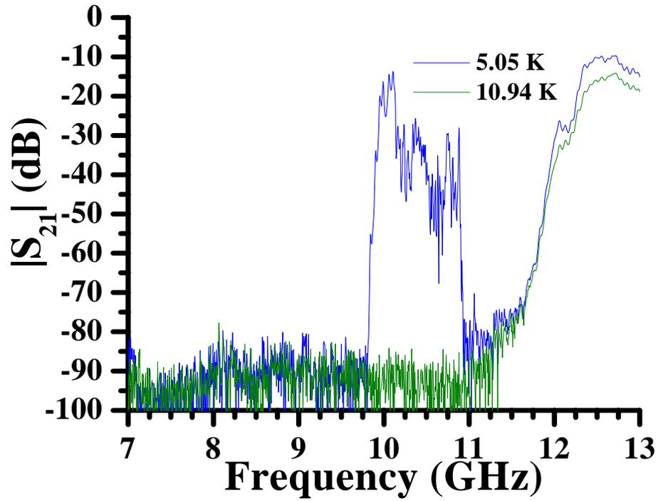
Figure 6.1: A plot of the electromagnetic transmission,  $|S_{21}|$ , versus frequency for an array of 216 Nb split-ring resonators in a Nb wire array measuring five wires transversely and eighteen wires longitudinally, with a lattice parameter of  $a = 5.08$  mm. The blue curve was measured at 5.05 K and the green curve was measured at 10.94 K. The distance separating the wires and Nb split-ring resonator was approximately  $d = 2.54$  mm.
