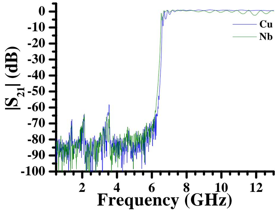
Figure 4.3: A plot of the electromagnetic transmission,  $|S_{21}|$ , versus frequency for an empty Ag-plated brass X-band waveguide, shown as a blue curve, and an empty Nb X-band waveguide, shown as a green curve. The data were taken at room temperature.
