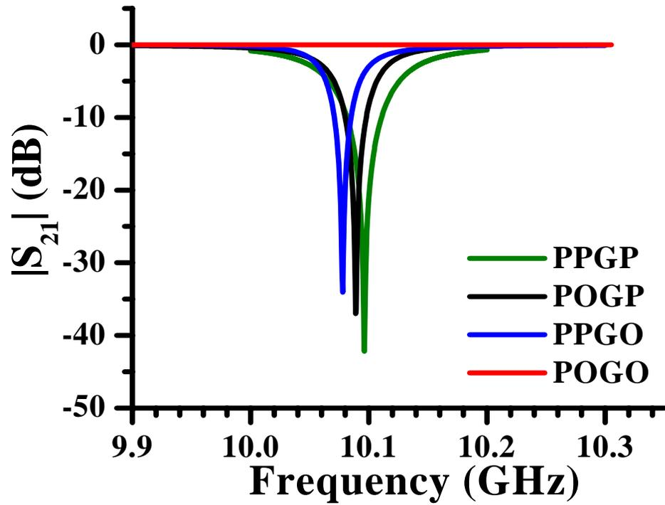
Figure 5.22: A plot of the electromagnetic transmission,  $|S_{21}|$ , versus frequency for a simulation of a single split-ring resonator made of a perfect electric conductor. The curves are labeled as follows: PPGO (blue): plane-parallel gap-orthogonal; PPGP (green): plane-parallel gap-parallel; POGP (black): plane-orthogonal gap-parallel; POGO (red): plane-orthogonal gap-orthogonal. The orientations were described in Figure (2.10).
