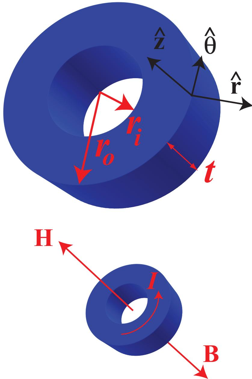
Figure 2.11: *Top*: A closed ring with inner radius  $r_i$ , outer radius  $r_o$ , and thickness  $t$ . The black axes show the cylindrical coordinate axes. *Bottom*: A closed ring with an applied magnetic field,  $\mathbf{B}$ , inducing a current,  $I$ , that generates an H field,  $\mathbf{H}$ .
