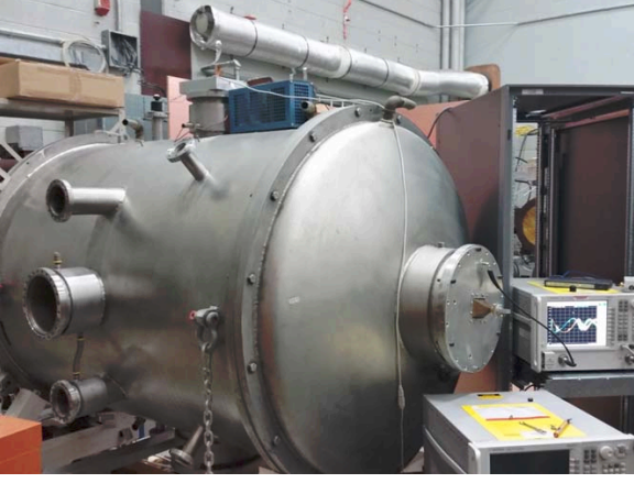
Fig. 6: The cylindrical stainless steel enclosure with a rotating mode stirrer
