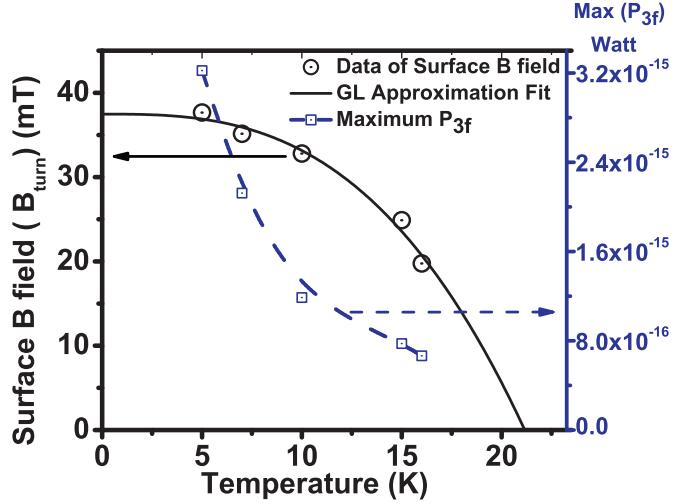
Fig. 6. Temperature dependent estimated surface critical magnetic field ( $B_{turn}$ ) of  $\text{Ba}(\text{Fe}_{1-x}\text{Co}_x)_2\text{As}_2$  and corresponding  $P_{3f}$  (indicated as  $\text{Max}(P_{3f})$ ) in Watts at the turnover point. Note that the dashed line is a B-Spline fit. The solid line is a fit of the surface critical magnetic field from Eq. (1), with  $T'_c = 21.15$  K,  $n = 2.88$  and  $B_0 = 37.47$  mT.
