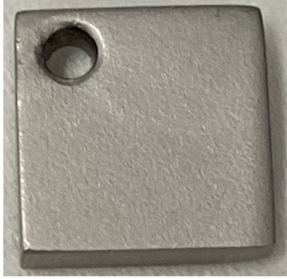
Figure E.1: Photo of the vapor-diffused \text{Nb}_3\text{Sn} film. The sample, prepared at Cornell University, has dimensions of 1\text{ cm} \times 1\text{ cm} .
