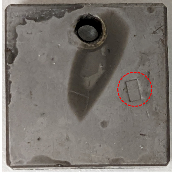
Figure E.2: Photo of the Sn-plated \text{Nb}_3\text{Sn} film. The sample, prepared at Cornell University, has dimensions of 1\text{ cm} \times 1\text{ cm} . The red dashed circle highlights a scar on the surface caused by an aggressive probe contact during a later measurement.
